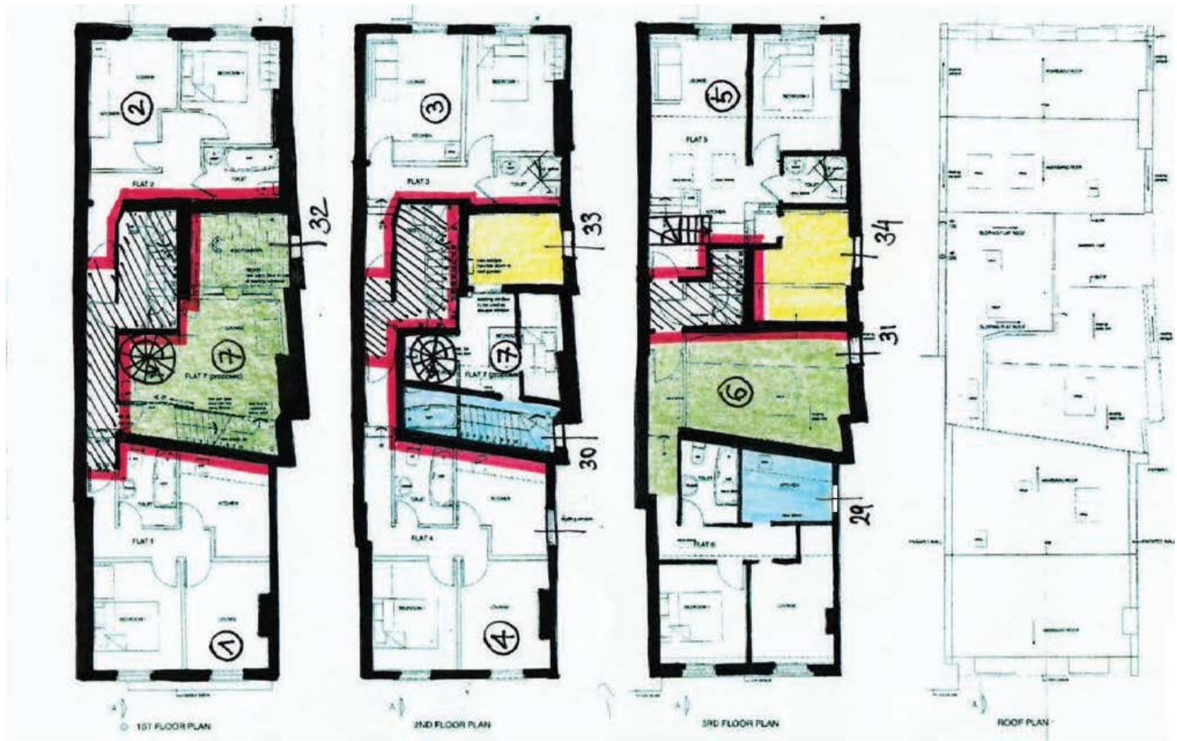
No.114 Peckham High Street. Plans showing internal layouts at 1st, 2nd & 3rd floor as built (flat Nos. 5, 6 & 7)
